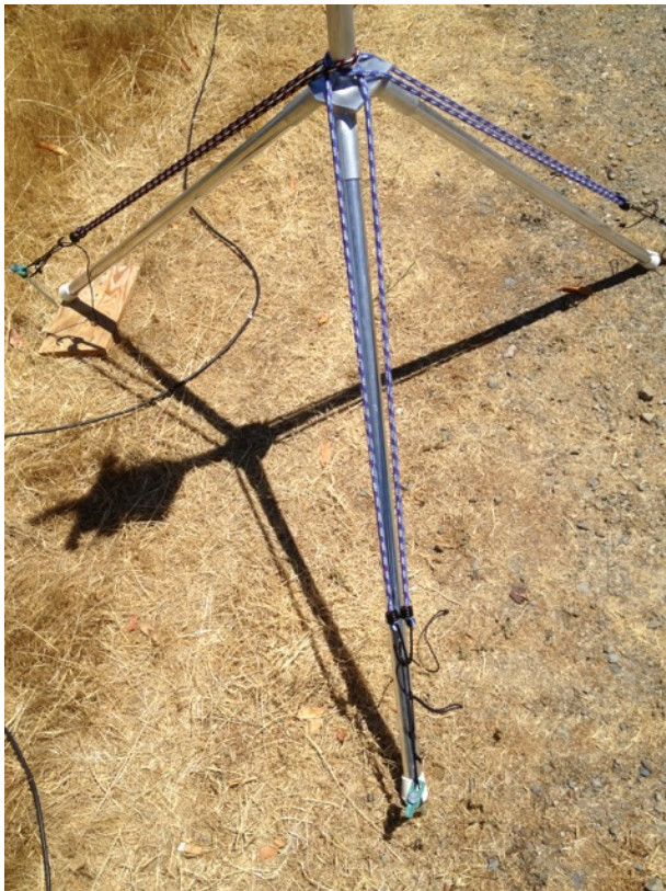
Figure 2. Tripod with elastic cords compressing the legs.
