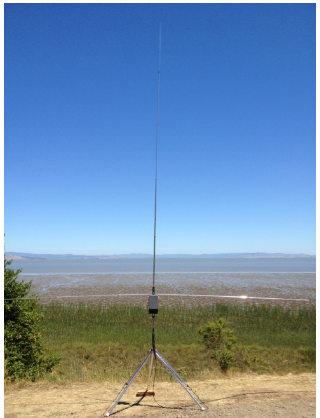
Figure 3. The modified 5k in operation, with the vertical element fully extended.
