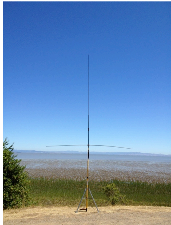
Figure 3. The Tinkertoy Vertical in operation, supported by a tripod secured with tent pegs.
