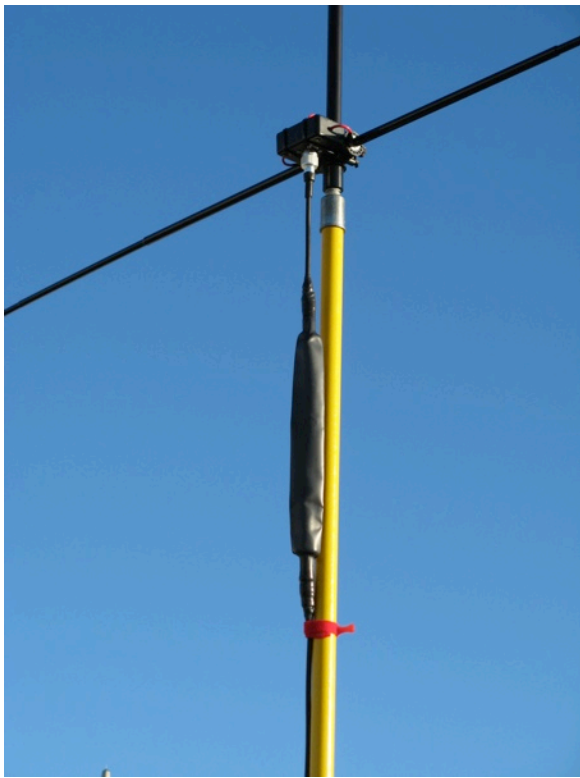
Figure 4. Close up view of the coax connection. The small project box is held to the back of the VersaTee using cable ties.
