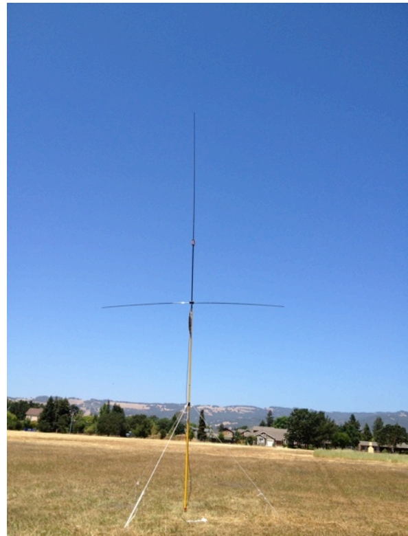
Figure 5. An earlier version of the Tinkertoy Vertical with a 12' painter's pole rather than the 8' one. The elevation is greater, but the band-change is more difficult. The antenna is supported here by guy ropes rather than a tripod.
